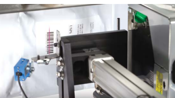
Continuous Print System verifies, folds and inserts Lit Packs
